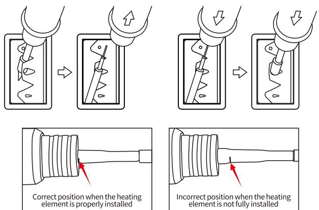
2. Connect the soldering iron and place the soldering iron into the soldering iron holder.
