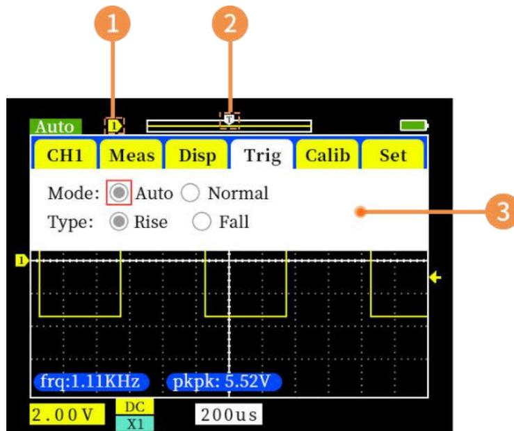
1.Switch by SEL button,Move the joystick up and down to move the vertical offset,Trigger position.
