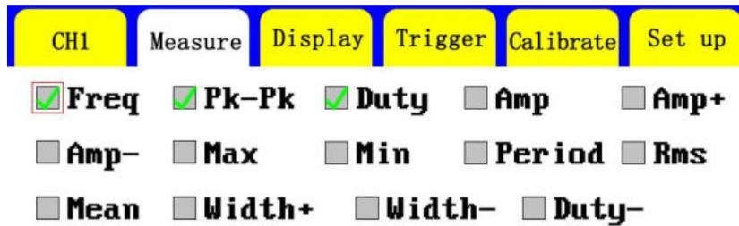
They are frequency, peak-to-peak value, positive duty cycle, amplitude, positive amplitude, negative amplitude, maximum, minimum, period, root mean square, average, positive pulse width, negative pulse width, and negative duty cycle
