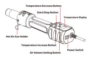
6-3. Press the temperature increase or decrease button to enter the measured temperature. Once done entering, press both buttons to confirm the entry and the system will automatically calibrate the temperature and exit the setting. - Setting complete.
