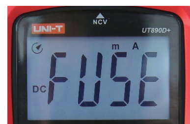
Fuse blowing alarm (mA only)
