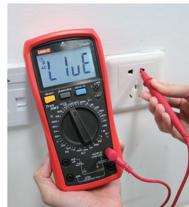
Live and nature wires identification
